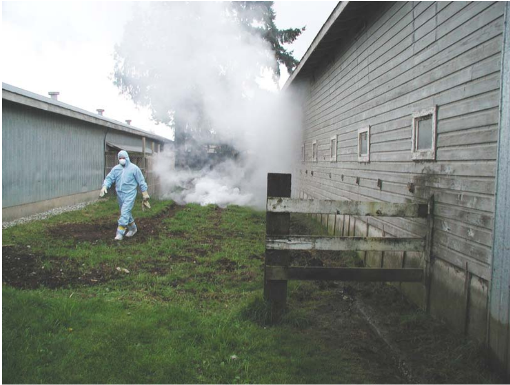
Figure 3. Demonstration of airflow characteristics using a smoke model
